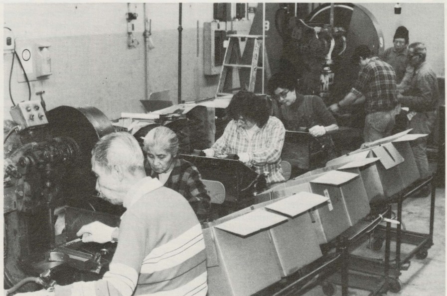
Assembling mobile home ventilators
